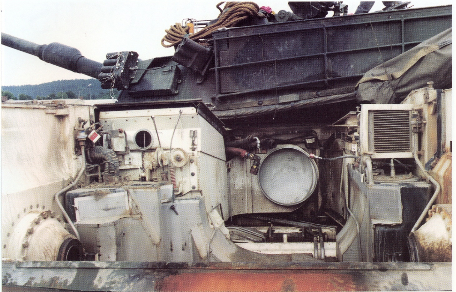
The empty engine bay seen from the rear. Note the heavy weathering from fuel, oil, and water. Of particular interest is the paint at the bottom, burnt away from the exhaust heat.
