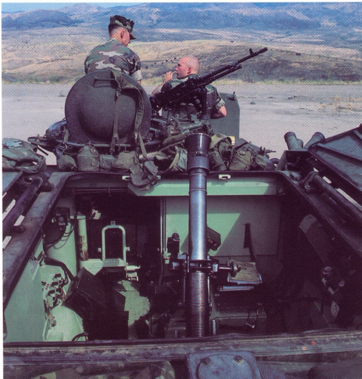
The top of the mortar LAV opens via three hatches to allow the barrel to elevate. It can also be rotated 360°. Five rounds of ready ammo is carried, along with 94 rounds in stowage.
