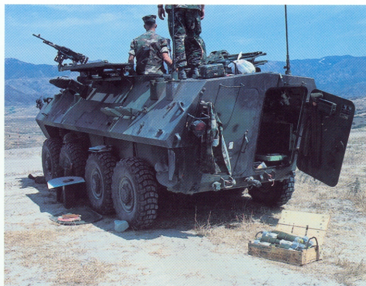
Top : In addition to its 81mm mortar, this variant has a 7.62mm machine gun with 1,000 rounds of ammo for self-protection.
