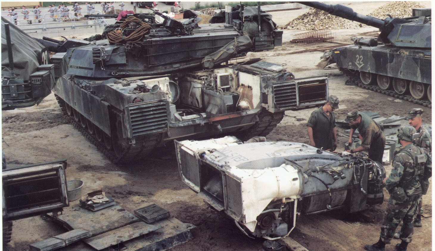
The empty engine bay seen from the rear. Note the heavy weathering from fuel, oil, and water. Of particular interest is the paint at the bottom, burnt away from the exhaust heat.
