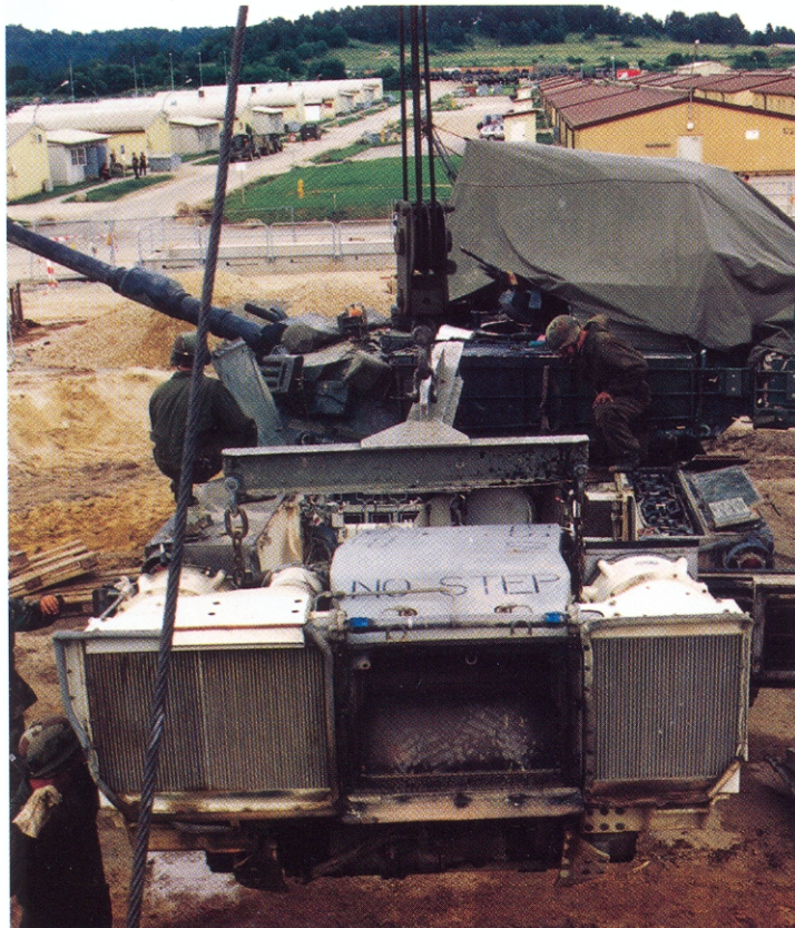
The engine deck, connected to a T-frame, is lifted by the crane of an M88 recovery vehicle.
