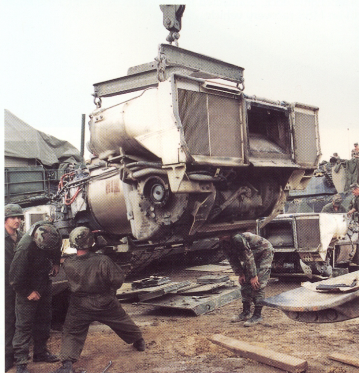
The powerpack is lifted by the M88, allowing maintenance to the underside.
