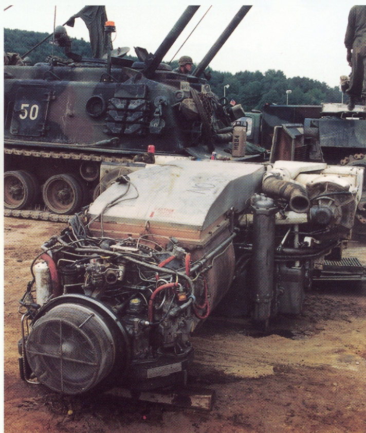
The M1 AGT 1500 Powerpack consists of turbine-engine transmission, final drive and cooling systems.
